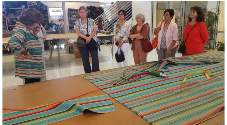
Ortiz-Spence (left) explains how the fabric is cut on large tables using electric scissors that can cut through several layers.
