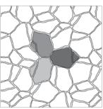
STEP 3 - Complete the balance of the surface to be covered with single pavers.
