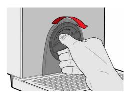
Align the shape on the inside of the filter cap (highlighted above) with the shape on the end of the new filter and push the two together until it clicks firmly in place.
