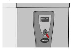
Grip cartridge and rotate a quarter-turn to the left and pull forward. CAUTION: A small amount of water will drain from the head.
