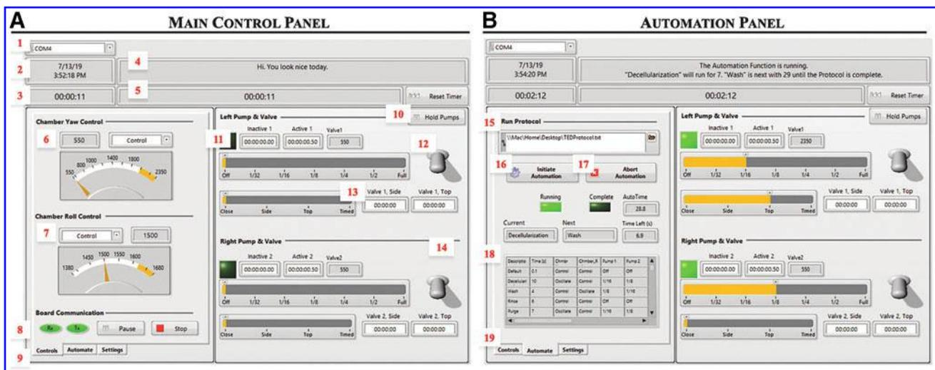
**FIG. 5.** (A) GUI of the LabVIEW VI written to control the TIPD in the Control panel. (B) GUI in the Automation panel, where a protocol for the automation of a process has been selected and initiated as shown by the Notifier (Callout 4) and the Automation Matrix (Callout 18). GUI, graphical user interface.
