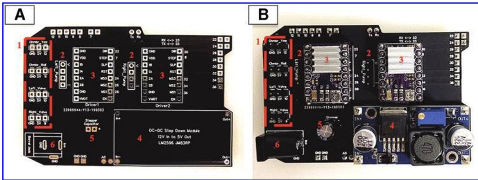
**FIG. 4.** (A, B) The non-populated PCB and PCB after soldering the requisite components, respectively. The six points of interest called out in the images denote the various pinouts, components, and modules necessary for controlling the device through Arduino-enabled microcontroller. PCB, printed circuit board.
