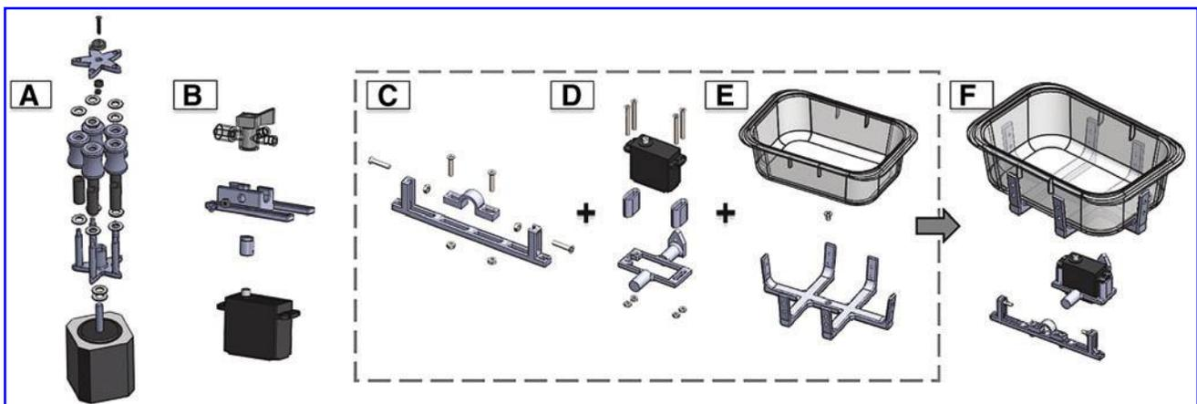
**FIG. 3.** (A) Exploded view of the Peristaltic Pump subassembly with a stepper motor at the base, driving the rotation of the pump once assembled. (B) Exploded view of the Valve Operation subassembly with a servomotor at the base, enabling valve selection within the 180° rotation range of the motor. (C–E) Exploded views of the *top-mount* chamber assembly. (F) The resulting subassembly of the *top-mount* chamber design.
