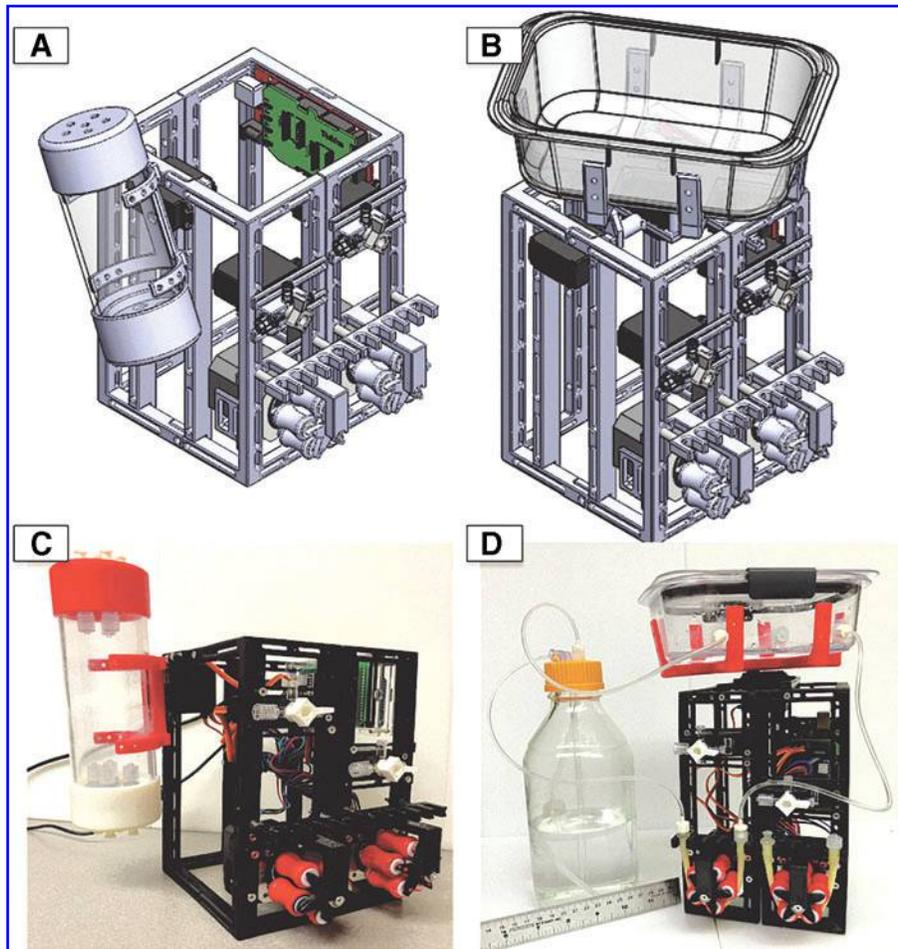
**FIG. 1.** (A, B) Solid Works CAD/CAM renderings of the TIPD with the *side-mount* and the *top-mount* chamber designs, respectively. (C, D) Designs after 3D printing and assembly of all components. For scale, a standard 1L glass Pyrex bottle is shown in (D). 3D, three-dimensional; TIPD, tissue infusion/perfusion device.
