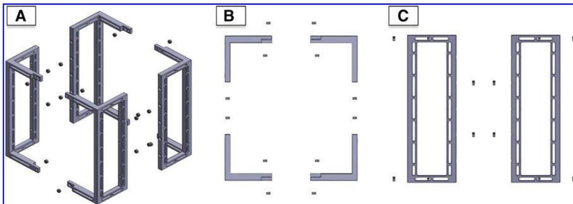
**FIG. 2.** (A–C) Exploded renderings of the Quarter Scaffold of the TIPD in isometric, *top*, and *front* views. In each image, sixteen  $6 \times 3$  mm magnets are exploded from the Quarter Scaffolds, where four magnets per part are press-fit for ease of dis/assembly.
