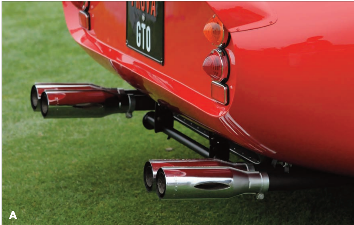
A. The glories of the iconic SNAP exhaust extractors as seen on the iconic 250 GTO.
