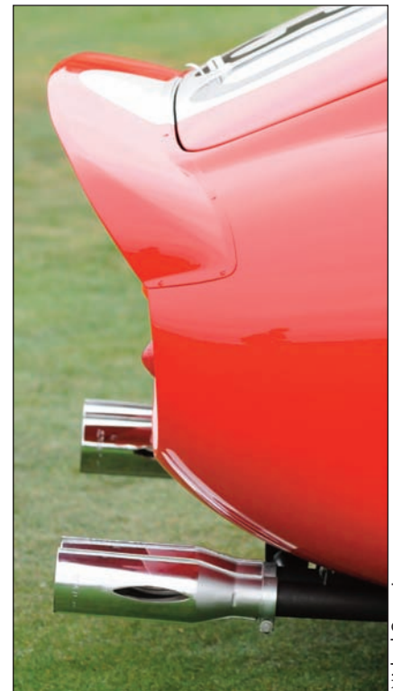
On the 250 GTO, the distance that the SNAPs extended beyond the body turned out to be a distinct advantage.
