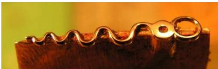
edges. Polishing can take an exceptional amount of time. When going from filing to the different grits of lapping film to the polish it is necessary to be certain that all the scratches from the previous level have been taken out
