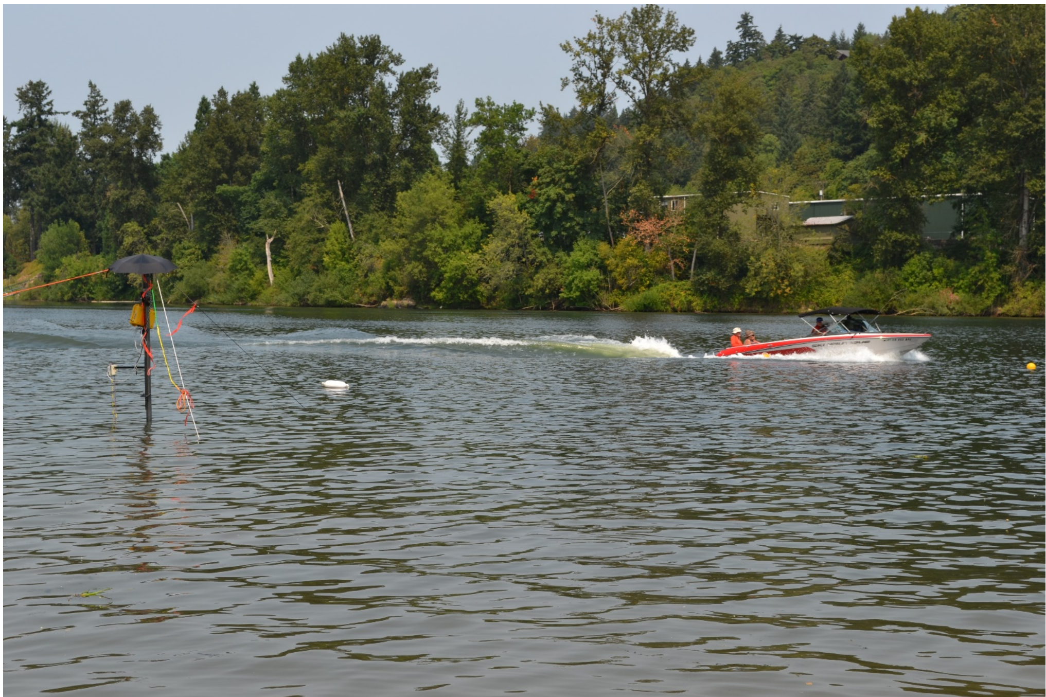
Figure 8 Photograph of 2015 Ski Nautique 200 at a speed of 12 mph and lateral distance of 100 feet (Run R70)
