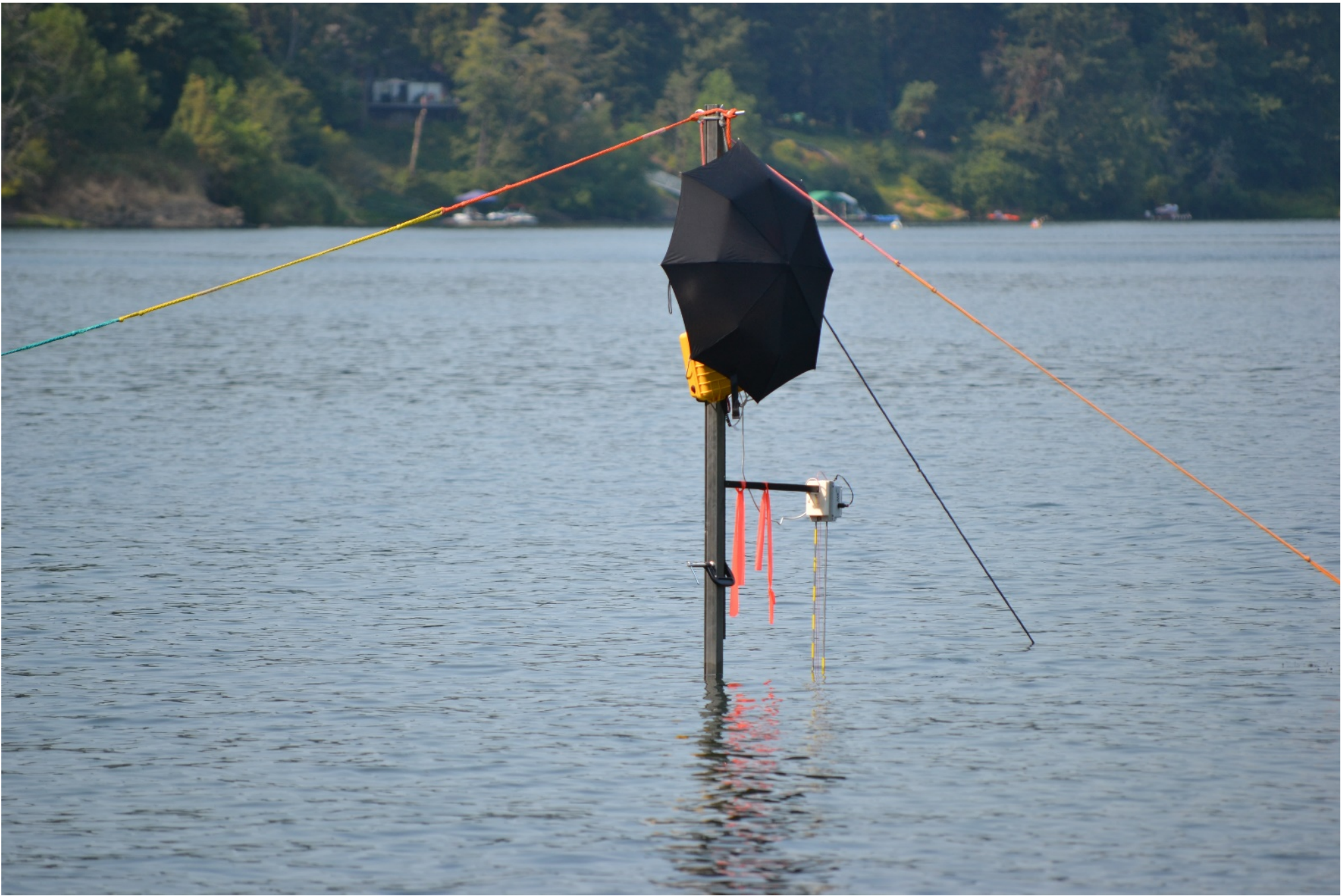
Figure 7 Photograph of the wave probe set-up
