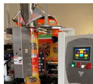
After - Upgraded Control Touch Screen with Start, Stop, Power and E-Stop
