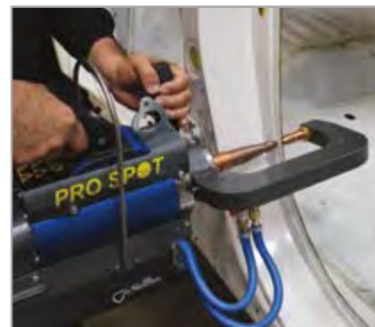
Spot welding of quarter panel using C-Arm.
