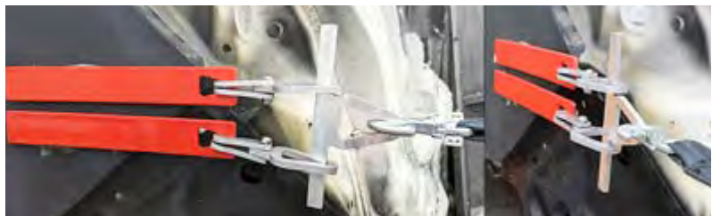
DENT PULLING WITH SCRAPE BARS
