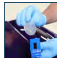
Plastic tabs are reusable and ready to pull dent after dent.
