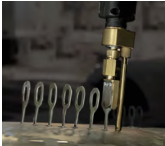
Apply keys and studs with Drawn Arc Welding
