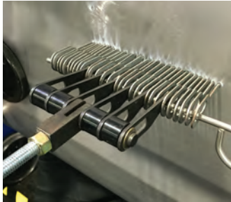
Tightly arrange keys for a more consistent pull
