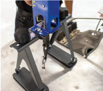
The PRO-65 provides targeted dent pulling
