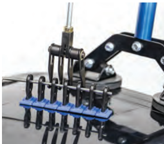
Quick and effective Paintless dent removal with the Glue Tab Kit and PB-10 Pull Bar
