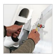
**1. BOLT REMOVAL** Remove the nut, bolt & washer from the vertical base walls.
