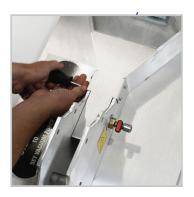
2. COVER REMOVAL Unscrew 4 screws to remove the venturi cover.
