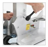
4. SECURE COLUMN Install the washer and nut onto bolt and tighten securely using a 17mm socket wrench and a 17mm open end wrench.
