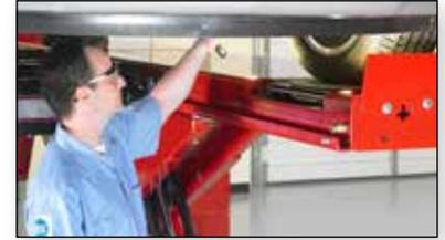
**H** *AlignLights turn on automatically at alignment height*
