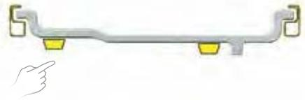
Rim cutaway displays selected weight mode
