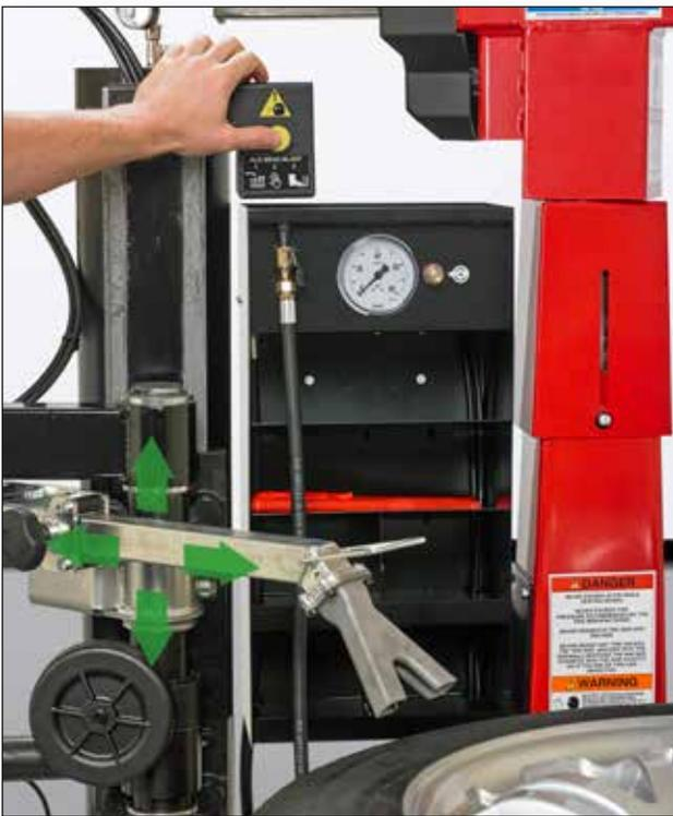
Large tank provides ample volume to seat the toughest tires. Simply set the position, select inflation mode then press the inflation pedal.
