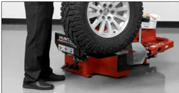
Optional wheel lift eases servicing of large assemblies. Allows for more careful handling of expensive wheels.
