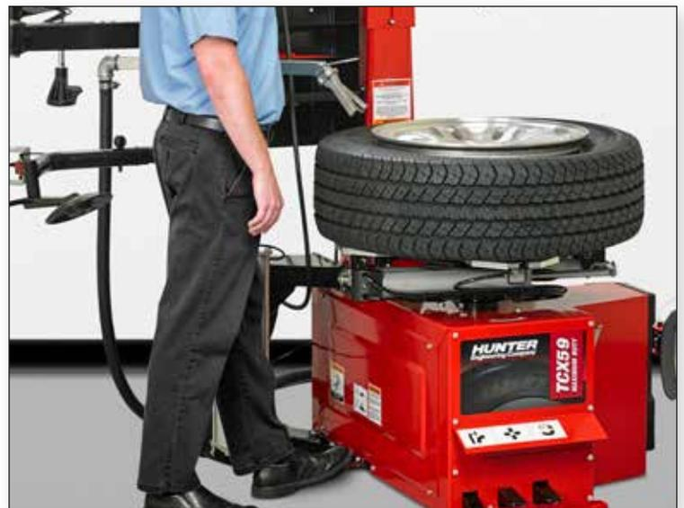
Nozzle is securely mounted to Bead Press carriage, allowing completely hands free operation.
