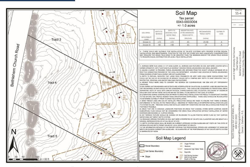
Note: The "+/- 1.0 acres" noted above on the soil survey represents the approximate area that was tested, which is the outlined area shown above listed with a suitability code of "A". This area is suitable for installation of a standard septic system.
