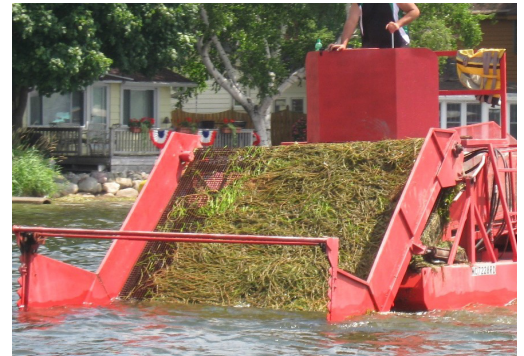
Vegetation removal in process
