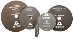
For certain applications, it is important to minimize the amount of damage done to the sample during sectioning. The AcuThin series offers thin blades that have been developed to minimize the area of cutting thus reducing the amount of damage to the sample. These blades utilize a rubber bond and allow for precise, delicate abrasive sectioning with minimal surface damage. [Blade Thickness is listed under Part Number]
