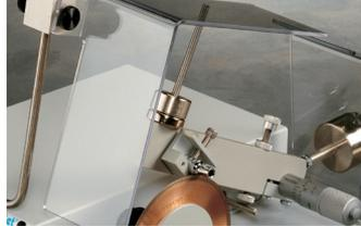
Prevents lubricant from splashing out of saw
