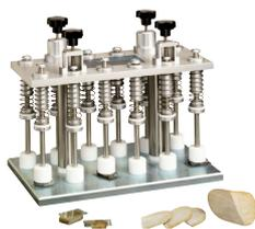
Assists in bonding specimens to glass slides, accurately controlling the thickness of the bonding media. Applies continuous pressure until sample has completely cured. Controls adhesive thickness by evenly distributing adhesive. Can hold up to 12 slides.
