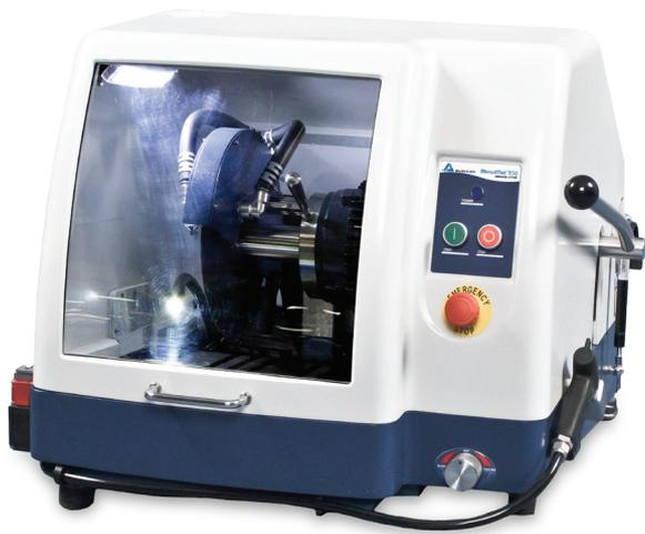
Allow for sectioning of parts with a 3.5in [88cm] diameter. (Varies based on part shape)
