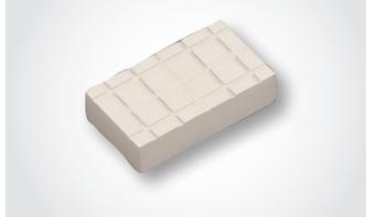
Use mounting wax, 40-8150 or 40-8145 to glue specimens to wafer chuck
