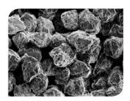
Angular, polycrystalline diamonds provide numerous cutting facets on the particle surface, resulting in less deformation.
