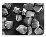
Sharp edges of monocrystalline diamonds ensure clean and efficient cutting action.
