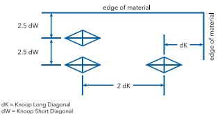
and the edge of a test piece shall be at least one diagonal (dK) or three and a half times the width (dW) of the indentation.
