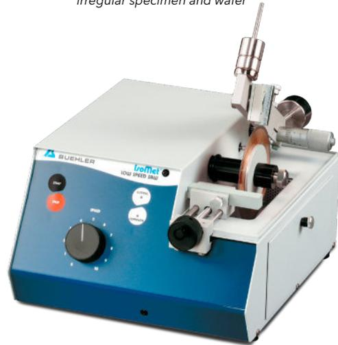
RPM ranges from 0-300 to provide cut quality for varied materials
