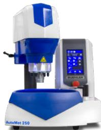
AutoMet 250 Pro has additional premium features. The enhanced programmability is highly intuitive with easy method storage. Improve repeatability with the automated dispensing system. The machine has z axis removal capabilities for grinding and polishing by depth.
