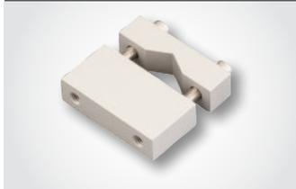
Medium Single Saddle Chuck holds up to 1in [25mm] specimen
