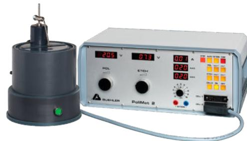
Includes controller, complete polishing cell and 4 masks
