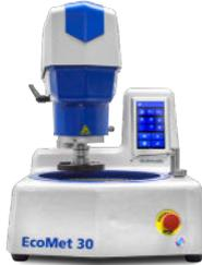
EcoMet 30 Semi-Auto is an entry level grinder-polisher with an emphasis on simplicity. All functions are easily accessible on an uncomplicated touch screen interface. It's compatible with a dispensing system to go hands-free during the polishing process and improve repeatability.
