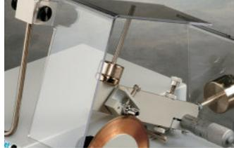
Prevents lubricant from splashing out of saw
