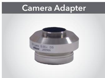
Camera Adapter, C-Mount, 0.55x, LV-TV, for 1/2" chip size cameras
