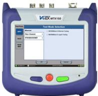
The MTX150 is a fully-integrated and self-contained multi-service test solution for OTN, SDH, SONET, PDH, DSn, C37.94, Ethernet, SyncE, Mobile Backhaul, and Fibre Channel (SAN). This all-in-one, rugged and ultra-portable field hand-held test set can be configured with interfaces and technologies required by field technicians to install, verify, maintain and troubleshoot Transport, Metro, Access communication links and services, including legacy applications.
