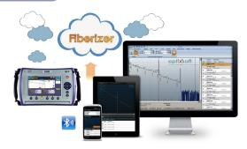
Fiberizer Desktop Plus is a standalone PC software application to analyze OTDR traces. Edit traces manually, create event tables, generate reports using built-in templates, and more.
