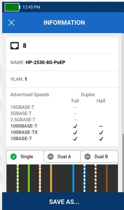
The LinkIQ-IE displays the switch name, port, and VLAN number in addition to the connection speed.
