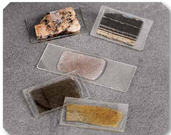
Mineral samples re-sectioned and thinned to 30 $\mu\text{m}$ .
