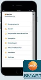
The App turns your smartphone/ tablet into the display for the testo 770-3. The display of the measured values are by Bluetooth® via the testo Smart App on your smartphone or tablet – irrespective of the measuring location. In addition, you can use the App to create measurement reports, add photos and comments to these and send them by e-mail. To ensure that your current clamp meter is always up to date, firmware updates can be carried out quickly and easily by connecting to the testo Smart App.
