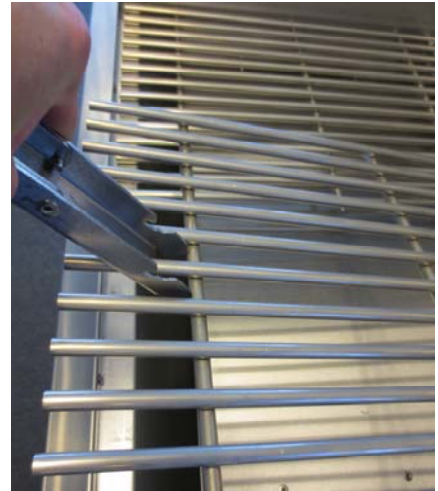
Step 1: Removal of the Grill Grates
