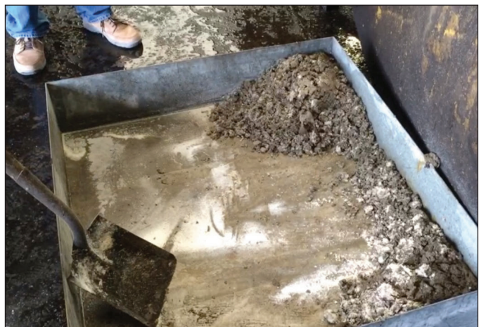
Liquid waste solidification using expanded perlite.
