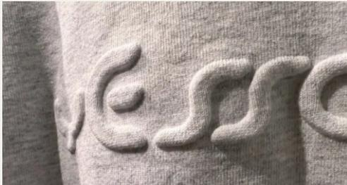
Embossing isn't ideal for small runs, as producing the metal die involves higher initial costs. However, the die can be reused over and over again - once created, it's suitable for thousands of impressions.
