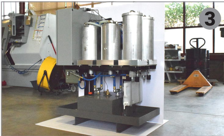
3. This custom skid-mounted Conserver® System is equipped with four HI4 purification units and two filter canisters. The unit is designed for systems with reservoirs or holding tanks up to 300 gallons. The system's unique control box measures flow, pressure and temperature, supplying the necessary logic and controls to ensure the unit performs properly.
