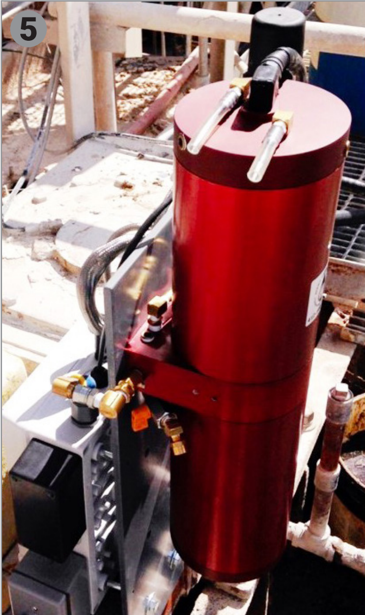
7. The HI2 Conserver® Oil Purification Unit installed on a lime kiln gearbox.
