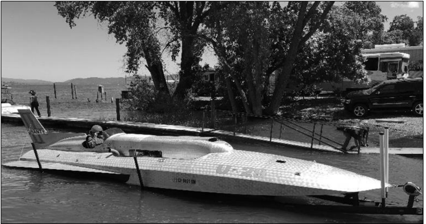
Steve Wilkie in his SHANTY II. Note the stabilizing wings near the cockpit. The boat was originally designed to bank into turns at high speed instead of sliding through turns like other hydros. The wings would prevent U-29 from flipping when banking. But secondary design changes made it impossible for U-29 to lean like a motorcycle, negating the need for the wings.
