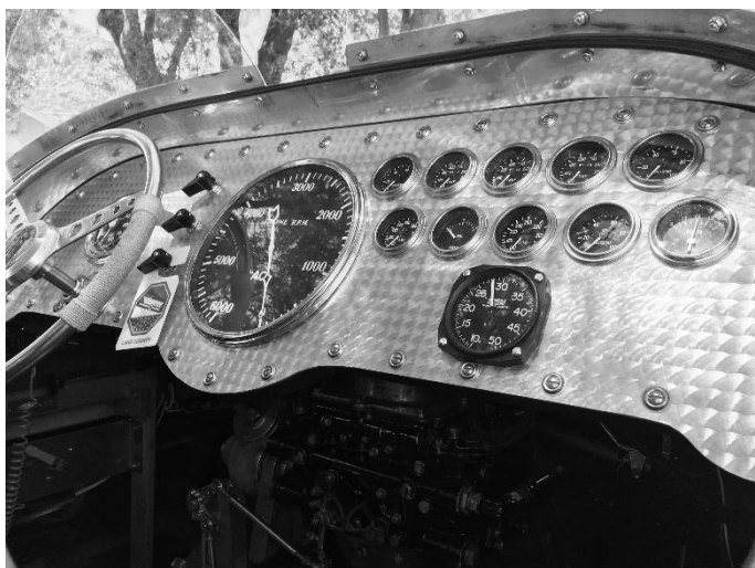
Note the rare, oversized tachometer on the NOTRE DAME's dashboard. It runs counterclockwise.
