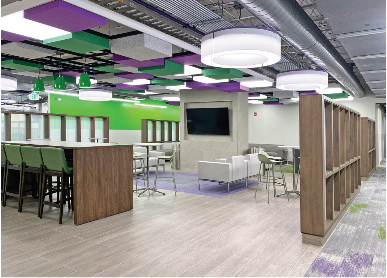
SOUND + COLOR At the training center's core is an open lounge area with a kitchenette and a variety of seating options for downtime between training sessions. A floating ceiling in the space serves to attenuate sound and conceal utilities, while adding visual interest.
