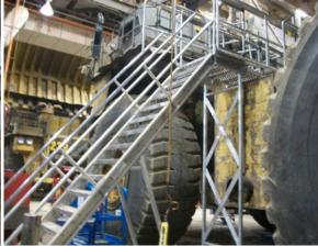
B&D Manufacturing's heavy-duty aluminum fuel tank stairs have the same characteristics as our aluminum manually propelled stairs product line, but with added features. This is the industry's first stair to safely allow access to the frame of many common haul trucks by way of a hinged boarding ramp that rests on the fuel tank.
