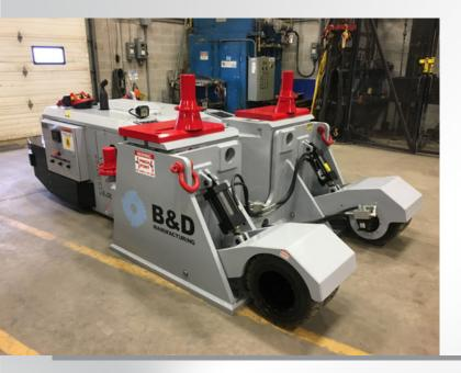
This equipment is the only certified two point lifting jacking system for the 240 ton to 400 ton (217 MT to 363 MT) Mining Haul Trucks.
