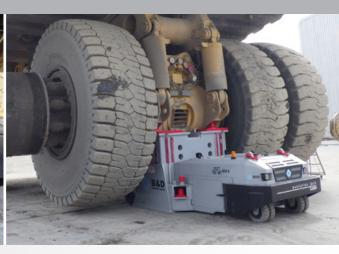
When maintenance is required on your fleet of Mining Haul Trucks, the B & D Evolution Jack can lift & secure the world's largest mining haul trucks. For excellent stability when removing and re-installing tires and wheel groups from trucks.
