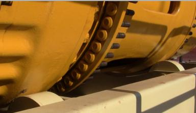
The Rear Wheel Group Removal tool attaches to the B&D Multi Handler cross slide assembly to install and remove truck wheel motor (final drive) assemblies.
