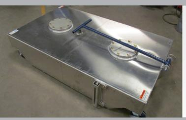
Constructed as a sealed and vented tank to reuse the antifreeze, our 140 gal (529 L) low profile cart comes with 2 in (51 mm) intake and discharge ports, 2 clean-out ports and sight glass. A heavy duty handle, four oil resistant swivel casters make it easy to maneuver. Fits under equipment of any size.
