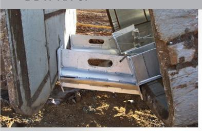
The B&D Dipper Door Safety Wedge is designed to secure the dipper door in place during maintenance activities.
