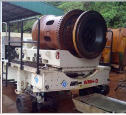
Increase safety, turnaround time and availability to your trucks using existing shop floor space. Designed for Caterpillar, Komatsu and Liebherr haul truck wheel motors, the B&D Multi Handler is Engineer certified and supported by B&D Manufacturing and distributors.
