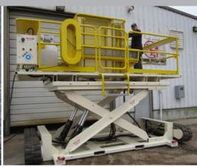
An easy, fast and safe way to replace and service the swing shafts for P&H 2300, 2800 and 4100 shovels.
