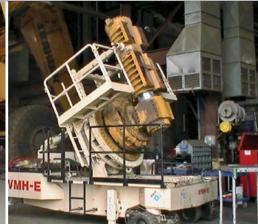
The Front Strut Removal Tool attaches to the main frame of the B&D Multi Handler to install and remove any model front strut (corner group) through the use of adapter rings.
