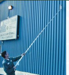
Made with lightweight, heavy-duty aluminum, spray can holders help mark out-of-reach areas, overhead and over holes.
