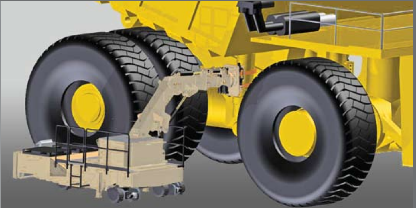
Pedestal Boom Removing Main Dump Body Cylinder
