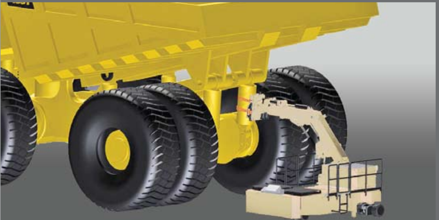
Pedestal Boom Removing Rear Strut
