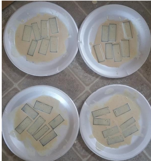
Figure 2. Seven clean and seven rusted cut pieces coated with NFRA 1 -base
