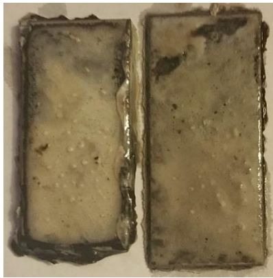
Figure 13. Day 7: Clean (left) and rusted (right) specimen after first cycle
