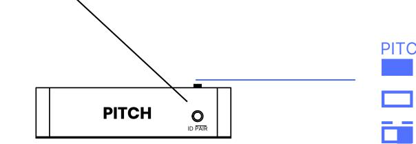
2. CANCEL EXISTING PAIR: While LED flashing hold button on Pitch for 3 seconds again.
