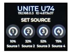
Rotate the controls to select the active Source for each Zone.
