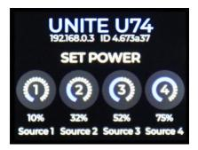
Each Zone can be individually powered-down. Rotate the Zone's control clockwise to activate, counterclockwise to power-down.
