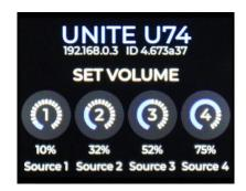
Rotate the controls clockwise to increase the Zone's volume, counterclockwise to decrease.
