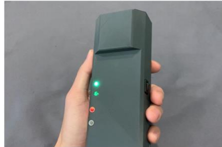
Current prototype of the POINTER receiver, which is worn by responders entering a structure. What is now the size of a cell phone will ultimately be reduced in scale and potentially integrated into existing firefighting equipment.
