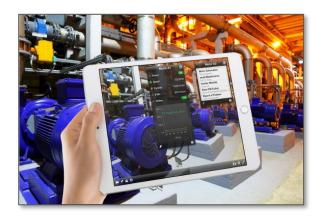
iQagent uses QR Codes (or your existing asset tags) to recognize equipment and process areas on your plant floor. We call these *Points of Interest*, or POIs. Our mobile apps scan these to display relevant data from your existing plant systems, including **live process data** from your PLC, HMI, or SCADA, schematics, documents, forms, videos and other resources from your existing PMMS and document management systems.
