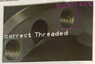
Monitor Quality: Absence of a real-time inspection data analysis system to monitor the process capability (Cpk) was resulting in defects and higher costs. The connected inline Statistical Process Control (SPC) solution from eMaestro now allows Omkar to automatically collect and analyze inspection data, view process status, trigger alerts, and initiate corrective actions based on predefined rules, in real-time. They can also review historical data for analysis.
