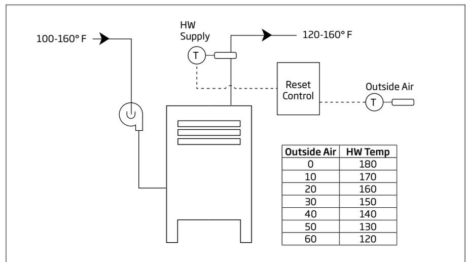
**Don't install a reset control on a boiler that's not designed to handle flue gas condensation.**
