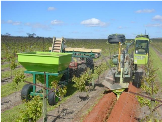
TG Drains can use different methods for delivering gravel into the machine's hopper depending on where the drainage is installed. For vineyards we use a gravel trailer with an elevator belt to bring the gravel up and over the rows of vines.
