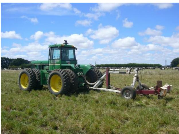
Mole channels must have an even, gentle grade, with minimal grade changes. TG Drains uses a floating beam mole plough to install the mole drains. A floating beam mole plough allows the expander to maintain itself at the set depth irrespectively of small ground surface irregularities and allows the ripperleg and the expander to produce a smooth gradient to the mole channels.
