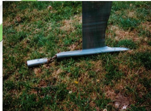
**Ripper leg with cylindrical foot and expander**
