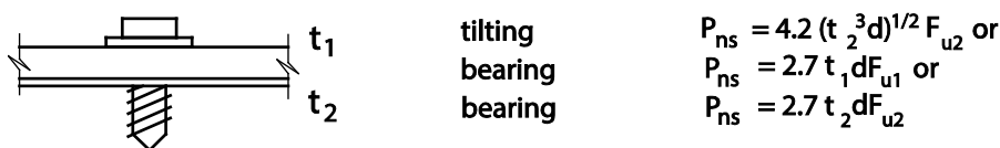
Figure C-J4.3.1-3 Design Equations for t_2/t_1 \leq 1.0
