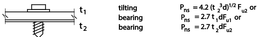
Figure C-J4.3.1-3 Design Equations for t_2/t_1 \leq 1.0
