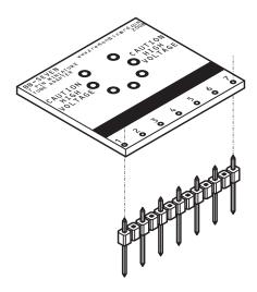
Align the seven pin socket (provided with the kit) with the hole pattern on the top of the board, insert pins through holes and solder.
