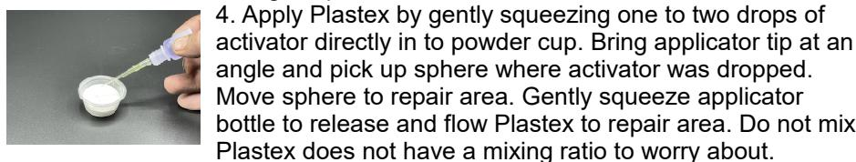
4. Apply Plastex by gently squeezing one to two drops of activator directly in to powder cup. Bring applicator tip at an angle and pick up sphere where activator was dropped. Move sphere to repair area. Gently squeeze applicator bottle to release and flow Plastex to repair area. Do not mix. Plastex does not have a mixing ratio to worry about.
