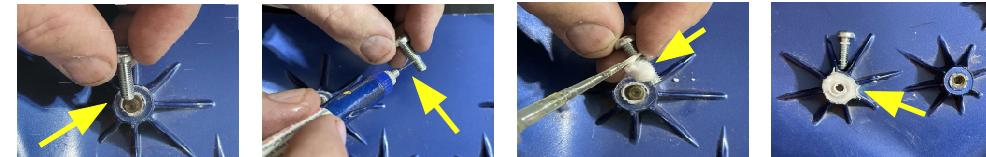
Ensure hole is slightly larger than the threads of the screw. Apply a thin coat of lubricant to the thread & wipe off any excess. Apply Plastex to the threads as needed and place coated screw in prepared hole, allow Plastex to cure. Then simply back out the screw. **TIPS:** 3-In-One Oil or oiling pen works best.
