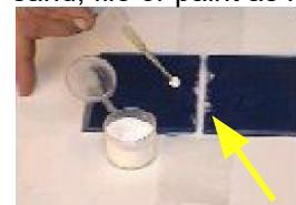
**TIPS:** Plastex cures in approx. 20-30 minutes @ 70°F/21°C. Thinner repairs or cooler temperatures will take longer to cure. Always make repairs as thick as base or original part. When possible always work from the back side to help reduce finish work of additional sanding etc.
