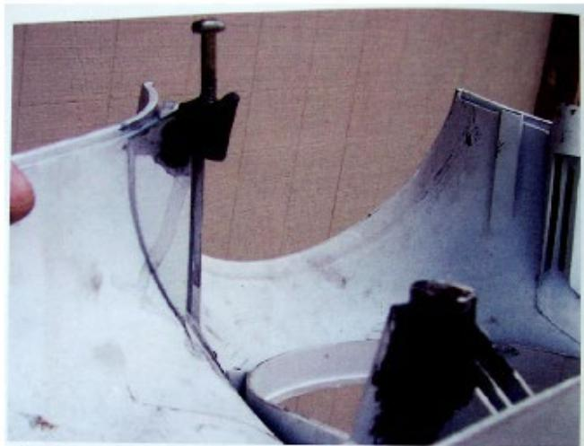
The underside of the headset was also missing a nut plate for attaching it to the underside of the headset. Previously considered lost forever, this piece can be replaced by re-creating it in Plastex. The process is a bit more difficult than just simple crack repair. It worked but was not as pretty as it could be.
