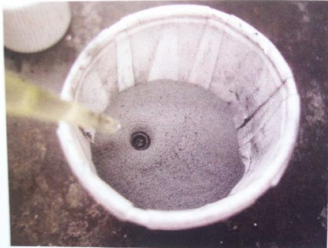
*Controlling the flow of the catalyst onto the plastic powder was tricky. After looking at the Tips section in the instructions, we realized the bottle should be nearly full, and we had very little product in ours. When the catalyst hits the powder, it becomes soft plastic and must be applied quickly.*
