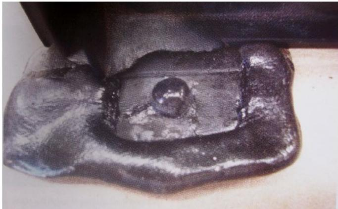
*This molding compound is supplied with the kit. It's heated to 120 degrees, then the broken part is pressed into the compound. Once the compound holds its shape, you stick the mold to the broken area and pour in the plastic powder with the catalyst.*
