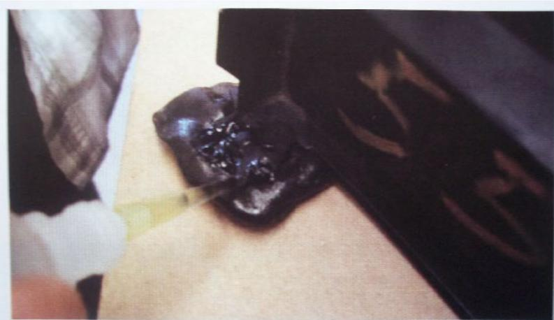
*We're applying the powder catalyst mixture into the molding compound. The trick is to keep it wet until the entire mold is full. As the powder is applied, additional catalyst can be applied to create a level surface. Be sure the powder is wet when it's applied against the original plastic.*
