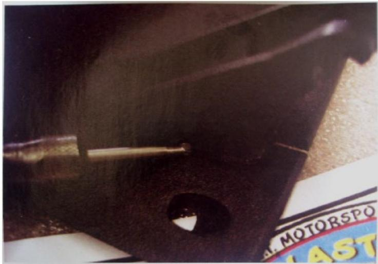
*If the area to be repaired has a crack, it must be opened up, leaving a "V" for the plastic compound to flow into and bond. You don't have to put the repair material on both sides. We used a Dremel tool at 600 rpm to limit the heat buildup so the plastic wouldn't melt during grinding. Cellophane tape can be applied to the backside of the repair to keep the Plastex repair material in place until it sets up.*
